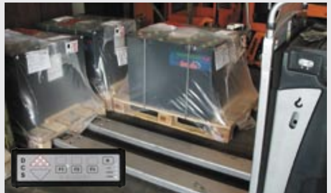
2-X fork (correct pick-up of a palette)
