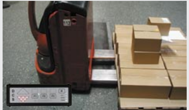
Lateral pickup, Europalette (truck – palette damage)
