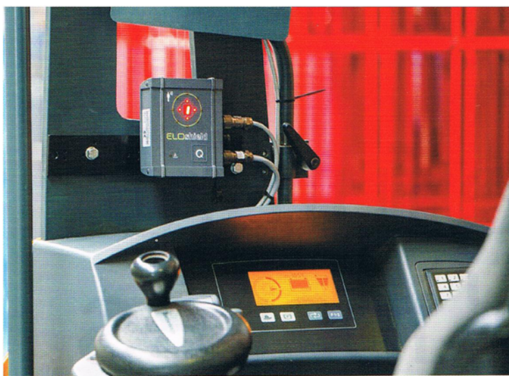
Mobile driver assistance systems can automatically detect the presence of personnel in a forklift's danger zone and send out warning signals.
