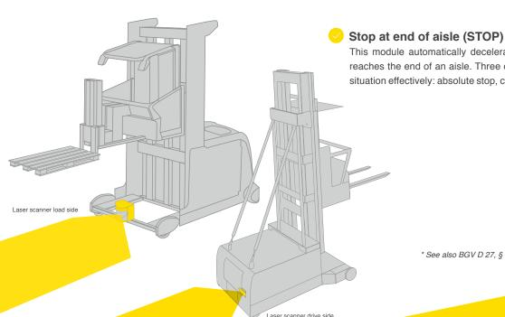
This module automatically decelerates and then stops a vehicle as it reaches the end of an aisle. Three options are available to manage the situation effectively: absolute stop, confirmed stop, and time-limited stop.
